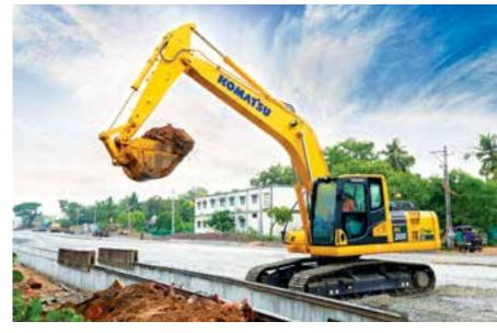
The fuel systems of these equipment are designed to work with B20 without any visible change in the performance and without altering the maintenance schedule. In addition, these machines can also run on 100% diesel without any modification, offering users flexibility along with quality, reliability and durability.
