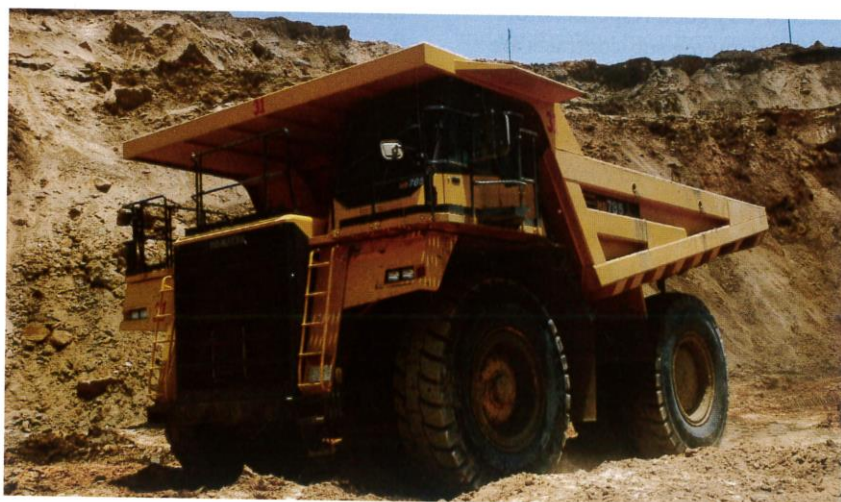
Komatsu HD785 dump truck, the most preferred off-highway truck in 100-ton payload in Indian market.
