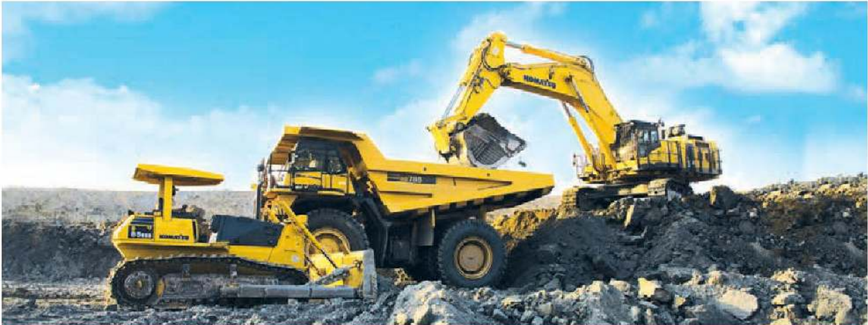
A spectacle of Komatsu machines engaged in mining project - PC1250 Hydraulic Excavator with HD785 Dump Truck and D85 Dozer.
