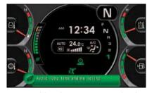
The ECO guidance menu enables the operator to check the operation record, fuel consumption history and ECO guidance record by pushing the button. The records can be used to reduce the overall fuel consumption.
